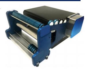
The Phoenix Autosampler's RFID system solves many of the issues of traditional NIR autosamplers by eliminating the need to track the order of samples or to follow worklists. The Phoenix Sideloader's autosampler system allows all sample information to be preprogrammed into RFID tags and analysis to be performed in batches of 30-50 or continuously by adding sample cups to the autosampler.
