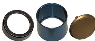
Small cups for ground and homogeneous samples
